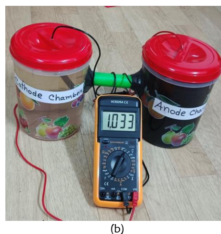
Figure 4: Design and assembly of the microbial fuel cell: (a) Schematic diagram of the dual-chamber MFC with electrodes, salt bridge and external circuit. (b) Photograph of the constructed MFC setup, showing the anode and cathode chambers, salt bridge, and electrical connections.
