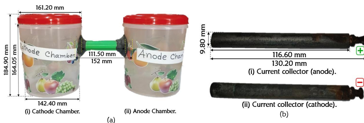
Figure 2: Structural components of the microbial fuel cell: (a) Dimensions of the anode and cathode containers. (b) Graphite electrodes as anode and cathode, with labeled dimensions and polarity.
