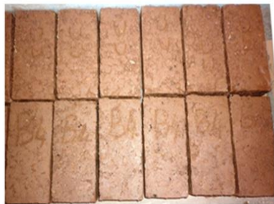
Figure 5: Curing blocks by air-drying
