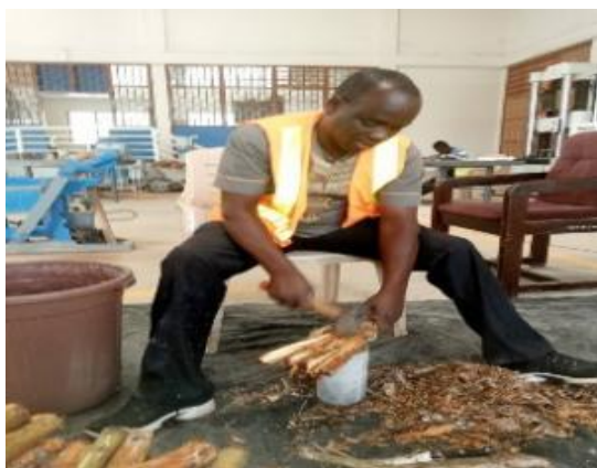
Figure 2: Hammering of stems to fibre
