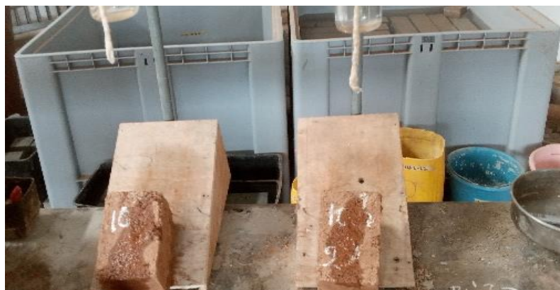
Figure 9: Simulated erosion test using the drip method
