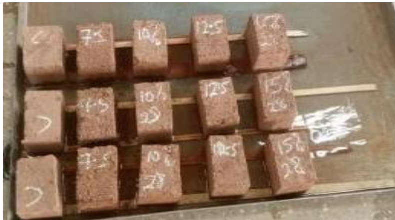
Figure 8: Water absorption of soil blocks by capillary
