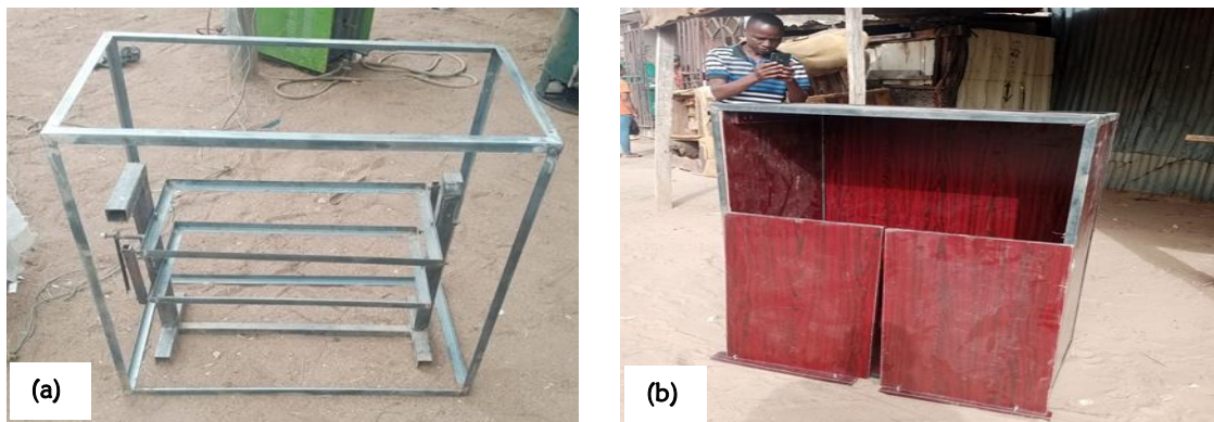
Figure 3: Skeletal view of the incubator (a) Metallic frame (b) cabinet frame
