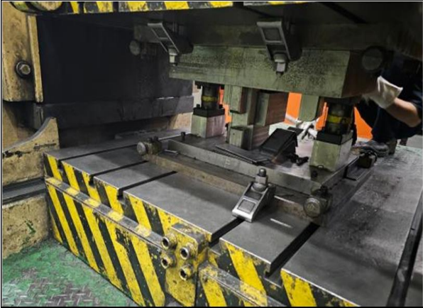
Figure 8: Completed die set for experiment
