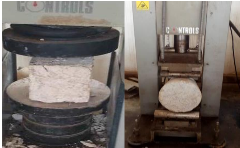
Figure 3: Cube and cylinder being crushed.
