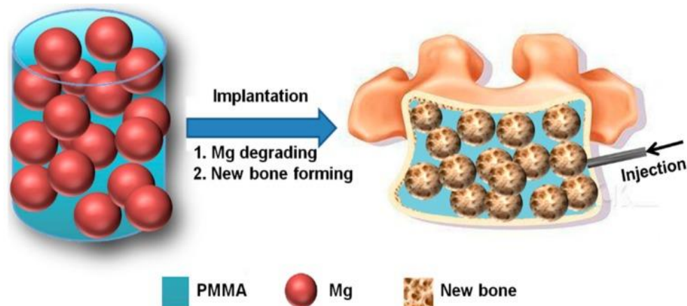
Figure 6: Schematic illustration of a partially degradable PMMA bone cement based on the “magnesium sacrifice” strategy. (Zhao et al., 2018)
