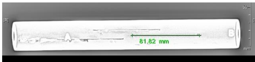
Figure 3: Defect Length of Radiographic Test Results
