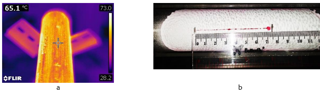
Figure 5: (a) Material image from the Flir camera (b) Defects produced at a surface temperature of 65.1 °C.
