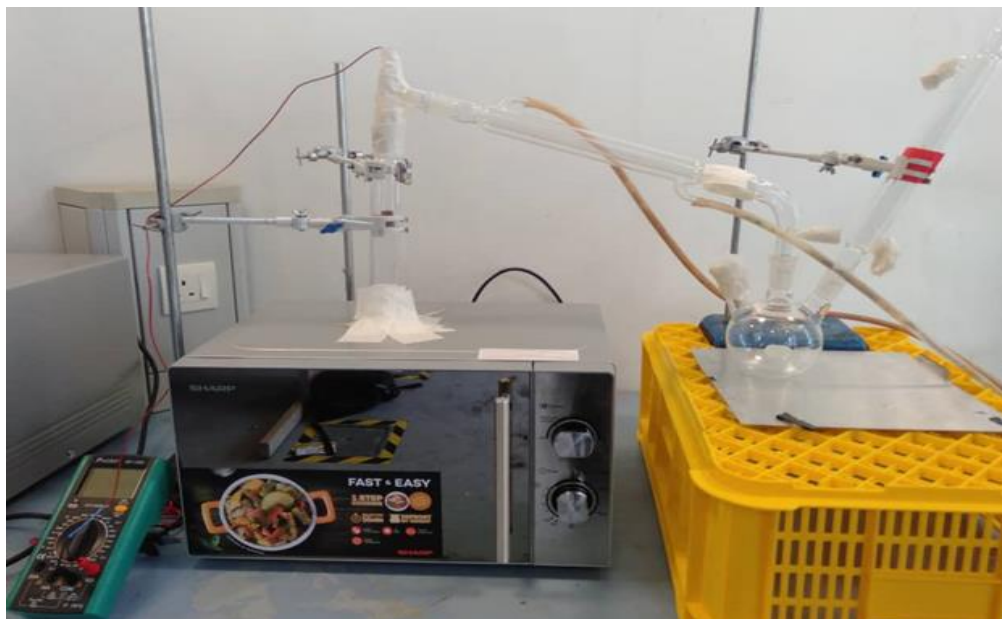
Figure 1(b): Modified microwave-assisted experimental set up for hydrothermal liquefaction process
