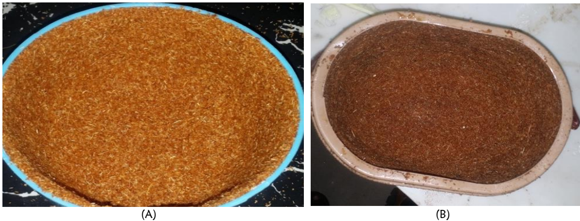
Figure 16: (A) Regency cooler filled with coir and bagasse and (B) Thermolineo cooler filled with coir and bagasse.
